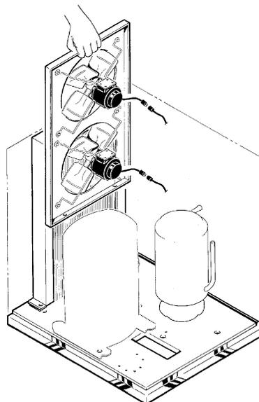
6. To reassemble: Place the fan motor assembly lower flange holes over the two allen head cap screws in the base, and reinstall the hex head bolts at the top of the assembly. Plug the fan motors back in, and replace the top panel.
