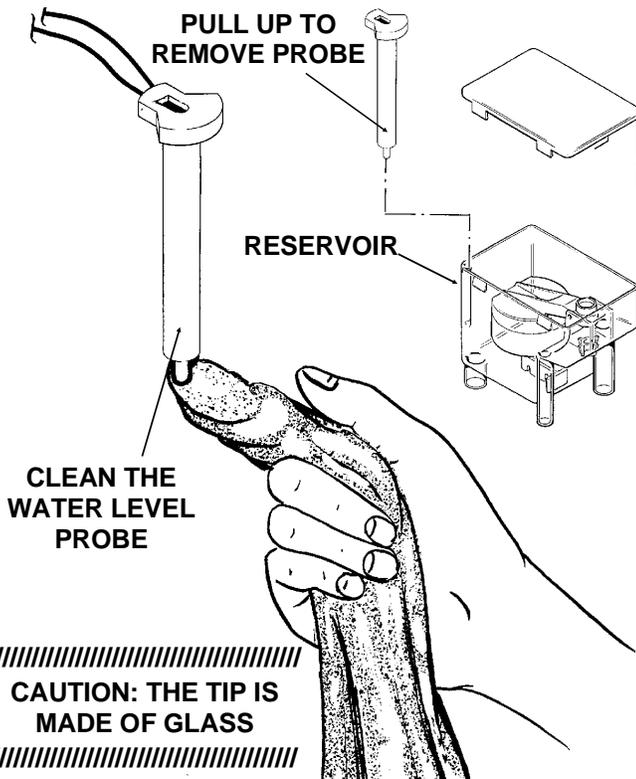
located in the water reservoir. At least twice a year, the probe should be removed from the reservoir, and the tip wiped clean of mineral build-up.
